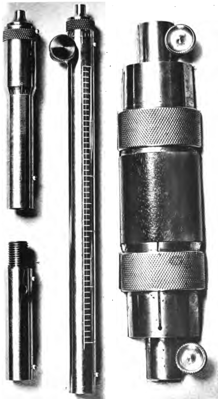
NO. 17. MICROMETER FOR INTERIOR DIAMETERS. RANGE, FROM 10 IN. UPWARDS.
